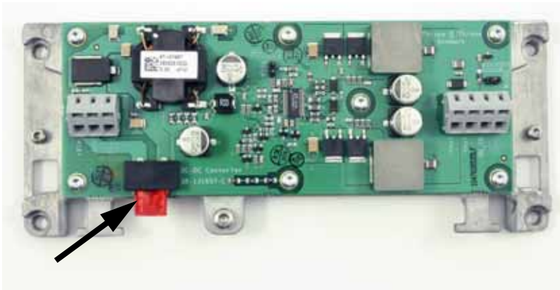
Figure 5: Replacing the fuse in the Power Converter
