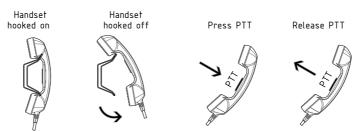
Transmit and receive is performed on the working channel shown in the telephone display. If the handset is used with an RT5020 duplex radio, received signal can always be monitored in the handset earpiece. With the RT5022 simplex/semi-duplex radio the received voice signal can only be monitored in the earpiece while PTT is released.
